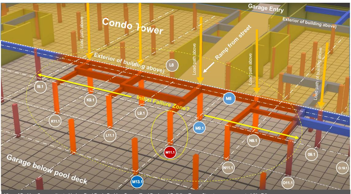
View of Parking Garage situated below Pool Deck. Parking Garage/Pool Deck and Building Tower Structure are connected (No EJ)
